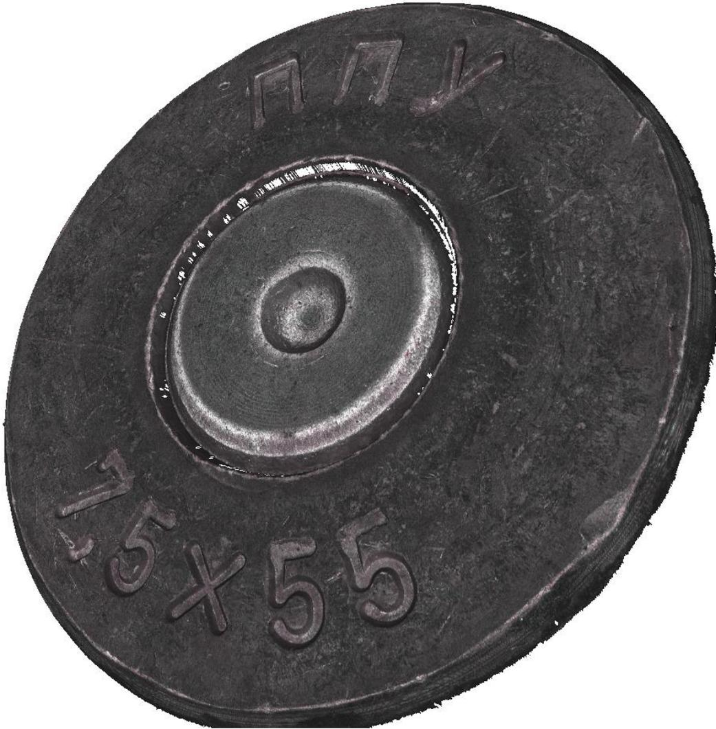
*Figure1: Head of a cartridge case acquired using the Alicona G5*
