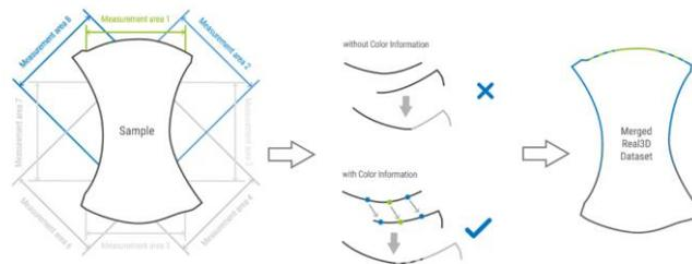
Figure 2 : Real 3D technology for complete measurement of the shape. The component is measured at different angles of rotation and tilt. A complete and precisely merged 3D dataset is created from individual measures that have overlapping areas.
