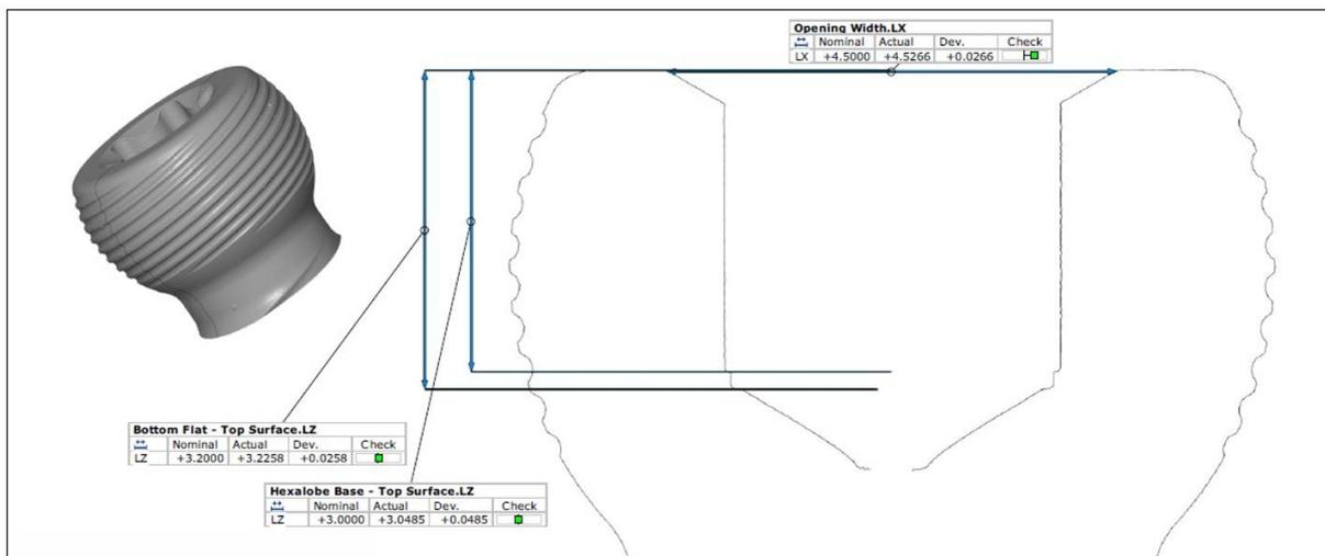
Figure 3 Measurement of heights and width inside the screw head
