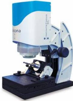
InfiniteFocusSL system with 50x50mm XY stage and fitted with rotation device. Info at <https://bit.ly/3sZS43H>
