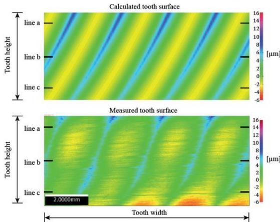
Calculated roughness versus measured roughness: The research team developed a mathematical model in order to investigate how machine parameters and possible error sources find their impact on the cut surface roughness.
