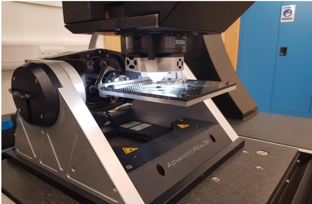
The specimen is a metallic and carbon fibre reinforced polymer (CFRP) stack, typical of assembly structures used throughout the aerospace industry.
