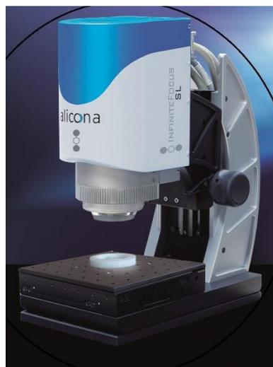
In use the standard flat coupon sample, as shown in Figure 1, is placed directly on the XY stage of the InfiniteFocusSL system, the stage on this system is able to move 50 x 50mm allowing large areas to be measured
