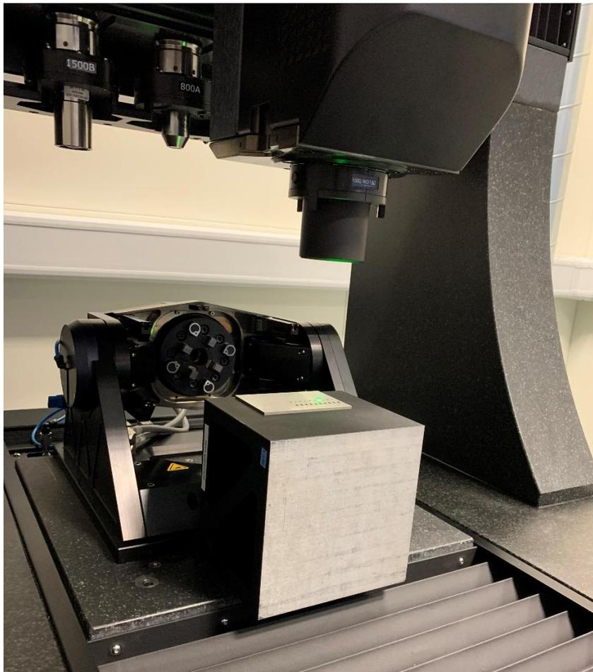
In this case a test plate with a series of EDM holes was created, illustrated in Figure 3. These holes represent typical holes used in cooling hole applications.
