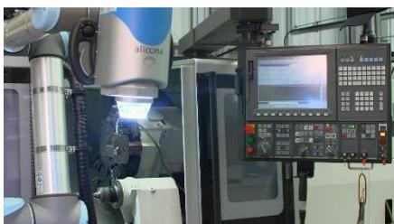
... and a further signal sets the Cobot in motion. The robot arm with 3D measuring sensor is automatically manipulated into the lathe...
