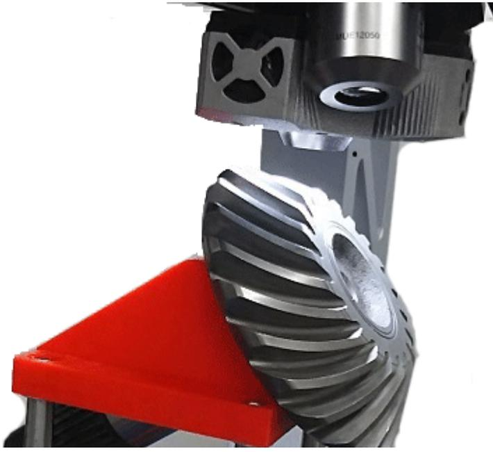
From this scan a 3D dataset of the tooth flank on either the pinion or ring as illustrated below.
