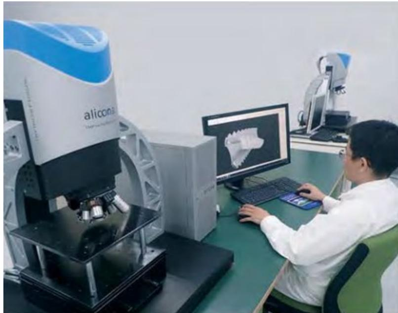
In use the gears are placed on the measurement platform and orientated to expose the surface to be measured, this can be carried out manually using the XY platform and motorised "Z" or with an optional advanced real3D unit providing a 5 axis automated measurement system.
