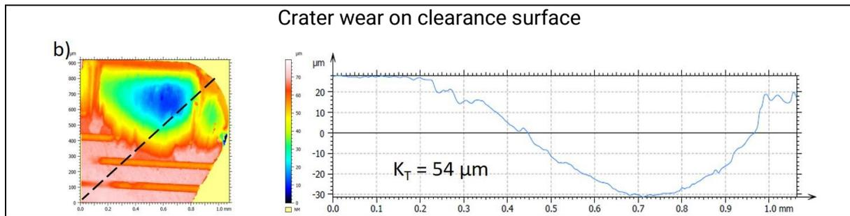
Figure 5: Acquisition and measurement of different types of wear on microtextured cutting tools (FEMTO-ST, Meliani, 2020)
