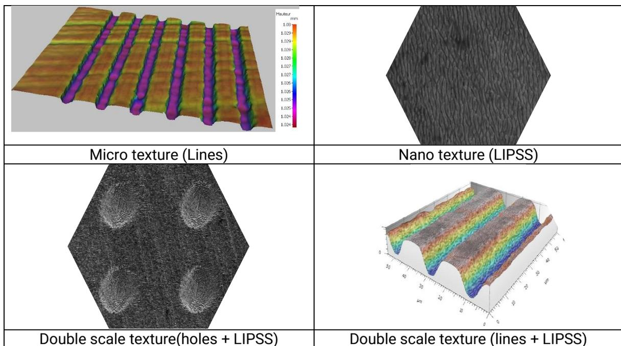
Figure 2: Topographic 3D view and SEM images of the produced textures (FEMTO-ST, Meliani, 2020)
