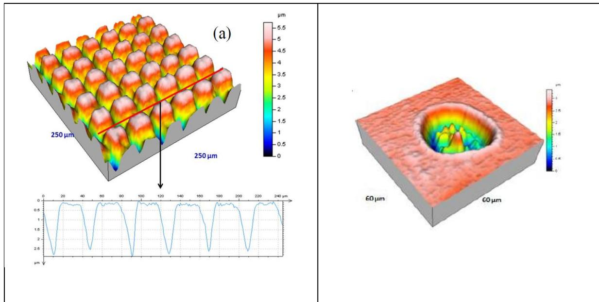
Figure 4: Topographic acquisition of laser microtextures (FEMTO-ST, Monteil et al., 2013)
