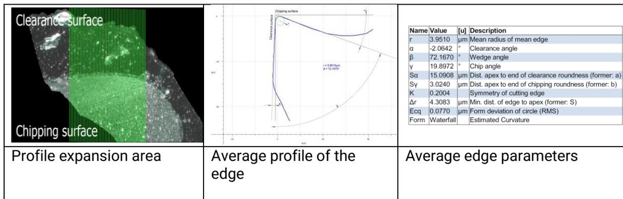
Figure 6: Acquisition and analysis of a cutting edge (FEMTO-ST, 2017).
