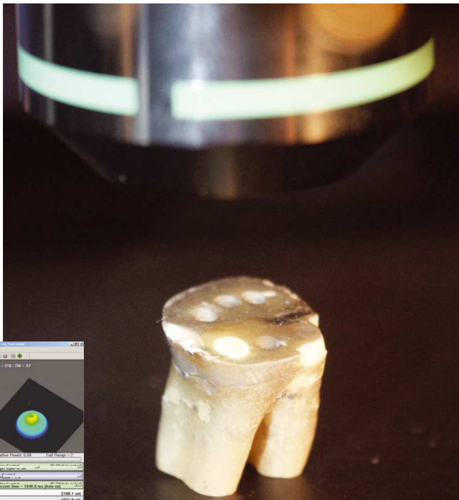
Infinitefocus Microscope (IFM) examining holes drilled in the test specimen. True-color images and volumetric measurements of the drilled holes assist researchers to understand the ideal energy distribution for an optimized laser drilling system.
